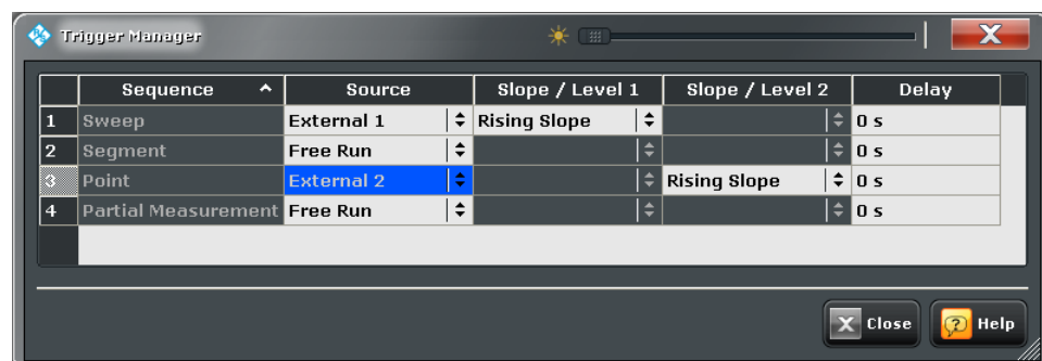
Figure 4-39: Example of a multiple trigger configuration
