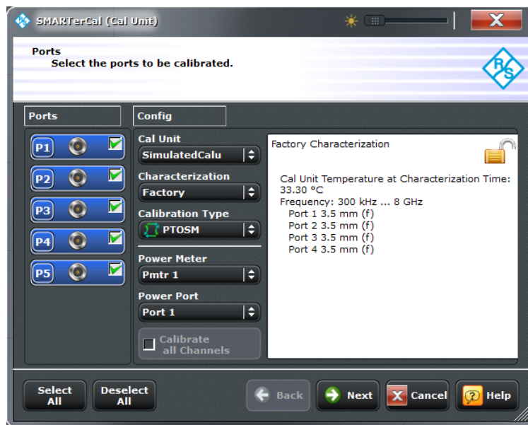
Figure 4-20: SMARTerCal setup (#Ports > 4)
