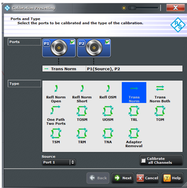
Figure 4-13: Calibration Presetting: Ports and Type
