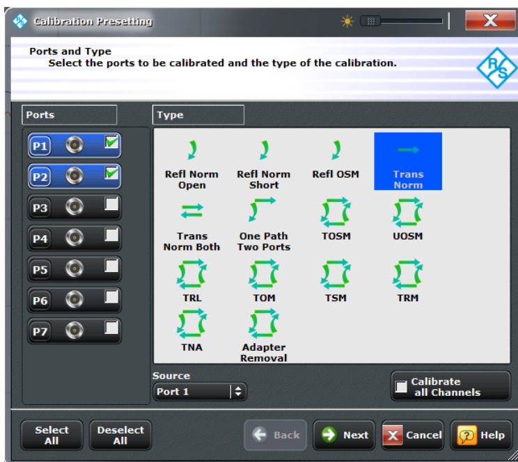
Figure 4-14: Calibration Presetting: Ports and Type (> 4 test ports)
