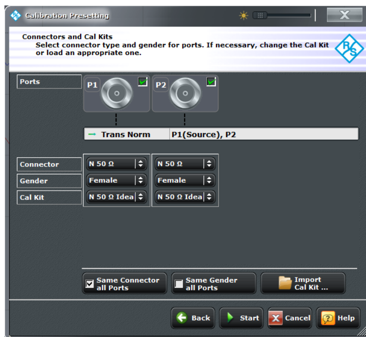
Figure 4-15: Calibration Presetting: Connectors and Cal Kits
